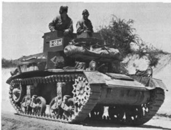
M2A3 light tank of the 68th Infantry at Fort Benning in 1940. The M2A3 appeared in 1938. Maximum armor was .75 inches and weight was 13 tons. Speed was 40 mph. Armament consisted of a .50 caliber machinegun in one turret and a .30 caliber in the other.
