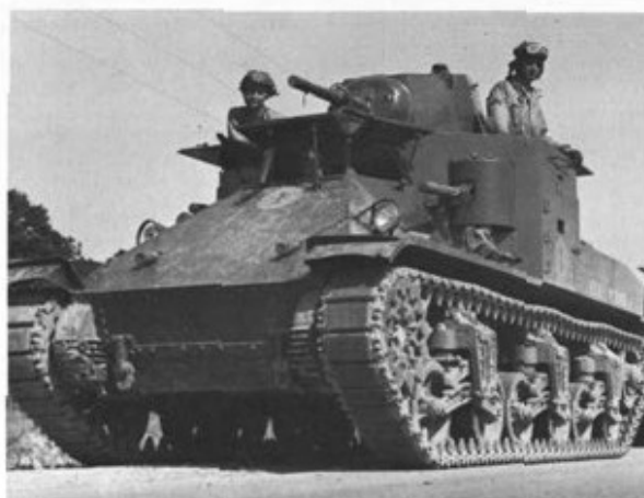
Production of the M2 medium tank began in 1939. A 350 hp Wright radial airplane engine pushed the 19-ton M2 to speeds up to 30 mph. Maximum armor thickness was 1 inch. Armament consisted of one 37mm gun and six caliber .30 machineguns.
